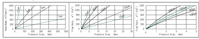
Please note the above Flow Rate is elements' co-efficient in cubic meters per hour per square meter. To get the flow rate of FT series filter, find the flow rate in the graph and then multiply it with effective filtration area on previous page.
