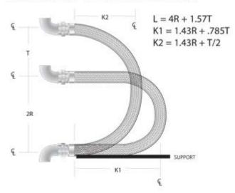
Note: In loop installations both connections and travel should be in same plane as the bend.
